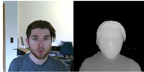
Figure 3.2: One sample pair of the captured depth dataset using a Microsoft Kinect v2 sensor.
